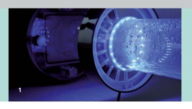
1 Demonstrator of the Nanopurhybridsystem consisting of microsieves and LED-disinfection
